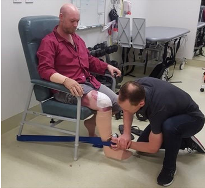
e) Traction belt over top of dynamometer, attached to anchor point on chair.
